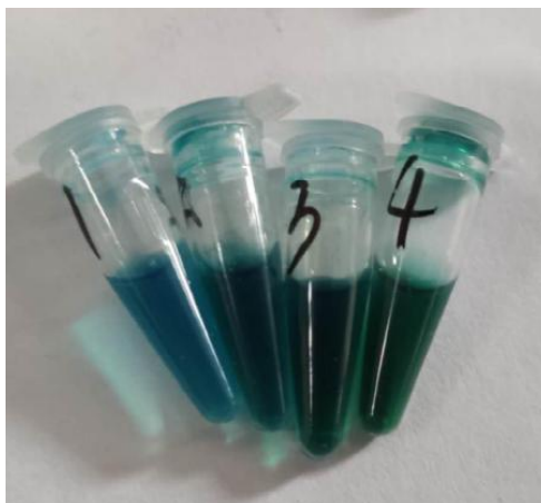
Figure 2: Color development of TMB induced by cerium oxide nanoparticles
